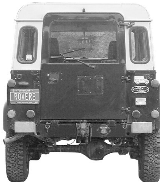
D90 with Rear Door #RNB037 without Spare Mount The difference between new rear doors is RNB037 has mounting facility for rear wiper and RNB032 does not. See page 60.
