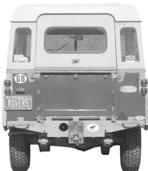
88" with Liftgate & Tailgate Liftgates, Tailgates and Rear doors can be adapted to all 88, 109, 90 and 110 models. See page 58.
