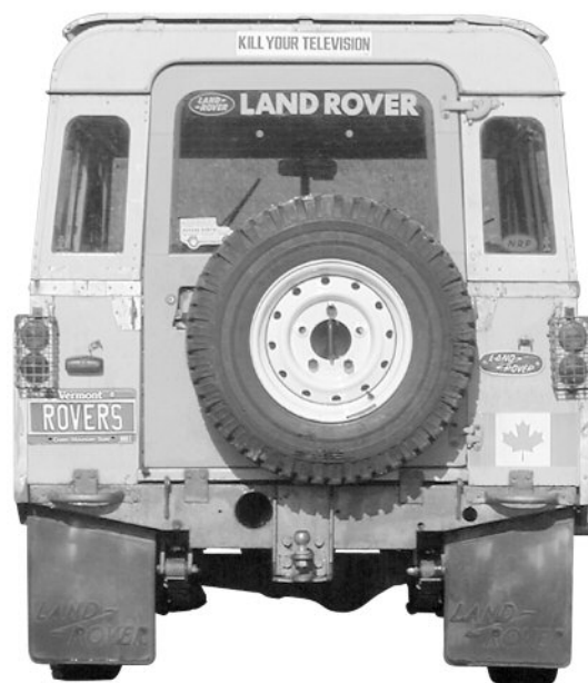
88" with New Genuine Rear Door #RNB032 Improved higher positioned spare wheel mount permits towing and improves ascent angles – see page 60.
