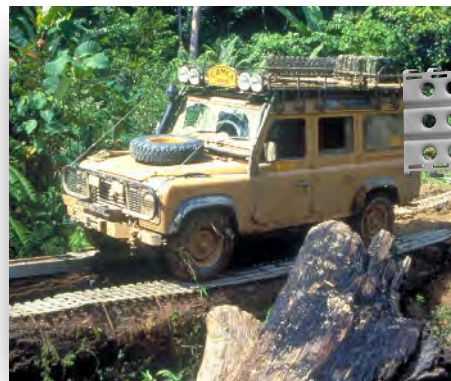
Defender 110 using aluminum platforms for traction over a log bridge.
