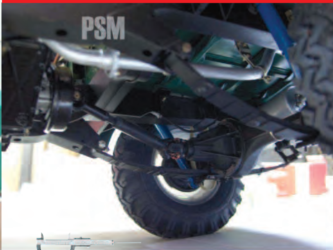
Functional front and rear suspension - very detailed brake assembly including wheel brake cylinder, brake shoes and springs. Wheels are fitted with real roller bearings.
