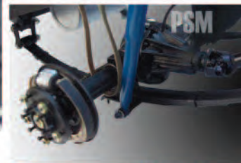
Functional front and rear suspension - very detailed brake assembly including wheel brake cylinder, brake shoes and springs. Wheels are fitted with real roller bearings.
