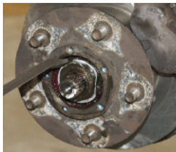
Fig 19 - The hub adjusting nut, lock washer and lock nut. Note that the tabs on the lockwasher are bent.
