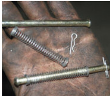
Fig 25, 26 - This is a close up of the rods and rod springs. Note the position of the pin in the end, the hole is sometimes hard to find. Above right is the caliper with new pads and brake grease installed.
