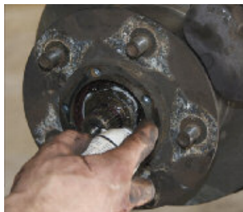
Fig 20 - Apply RTV silicone sealant (or similar) to the drive member hub face only before applying gasket.
