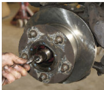
Fig 16, 17 - Grease stub axle before putting hub-disc back into place. Remember to hold caliper to side when fitting hub-disc assembly. With the caliper in hand, get a feel for the tension of the brake lines. Be very careful not to put stress on the brake lines.
