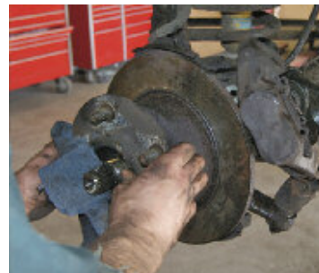
Fig 5 - Pulling hub-disc assembly. Hold caliper to side, put back in place after removing hub-disc assembly.
