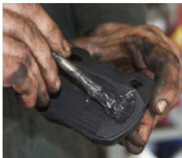
Fig 29 - Apply brake grease or copper anti-seize on the back of the pad. To avoid it rubbing off onto the piston, try to slide pad in with as much room as possible. This is done by working the pad back and forth to fully depress caliper pistons. Applying brake grease will not work if the piston scrapes it all off during the install.
