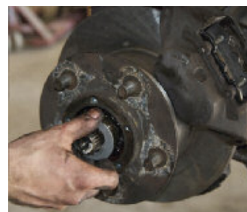
Fig 18 - After the outer wheel bearing, install the hub adjusting nut, lock washer and lock nut.
