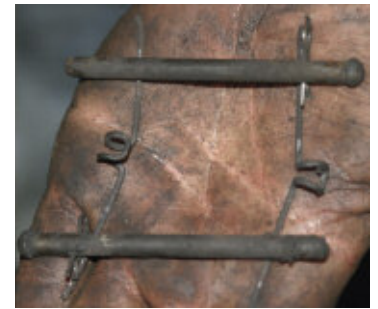
Fig 23, 24 - The caliper before removing old pads and pins. Above right is the pin and tension spring as they should look when put back together.
