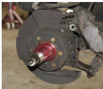
Fig 16, 17 - Grease stub axle before putting hub-disc back into place. Remember to hold caliper to side when fitting hub-disc assembly. With the caliper in hand, get a feel for the tension of the brake lines. Be very careful not to put stress on the brake lines.
