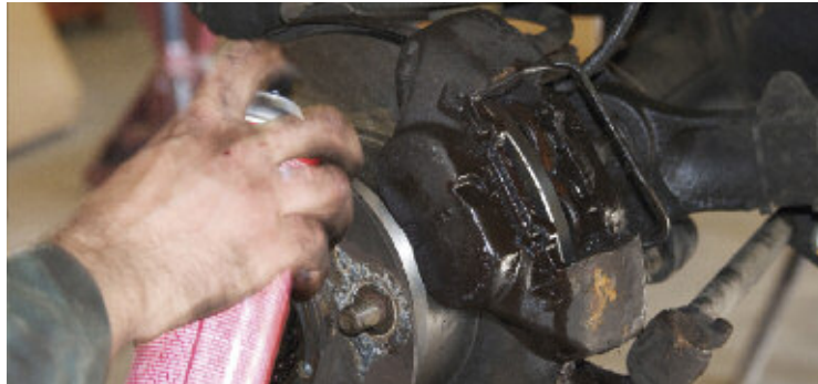
Fig 27 - Clean the disc, caliper and complete assembly with a brake cleaner.
