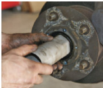
Using the hub nut removal tool RNF406.
