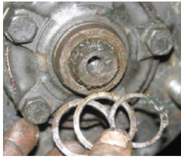
Fig 22 - The two driveshaft shims and circlip, with drive member installed and tightened.
