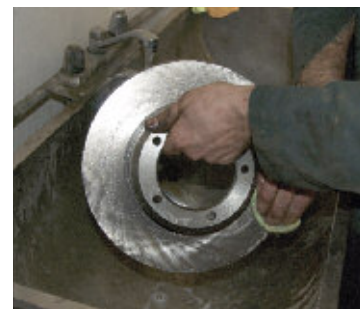
Fig 12 - Before assembling disc to the hub, clean with hot soapy water to remove any protective manufacturing film.
