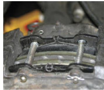
Fig 25, 26 - This is a close up of the rods and rod springs. Note the position of the pin in the end, the hole is sometimes hard to find. Above right is the caliper with new pads and brake grease installed.
