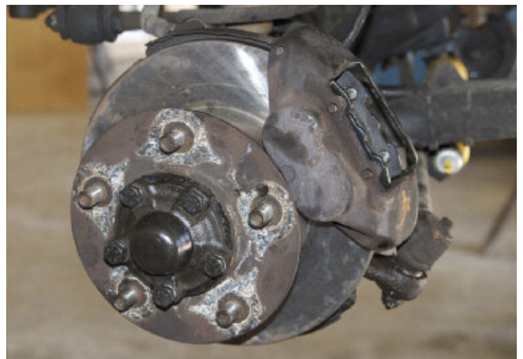
Fig 30 - Finished brake disc install. Clean any small grease or residue off with brake clean again, keeping care not to get any on the brake pads.
