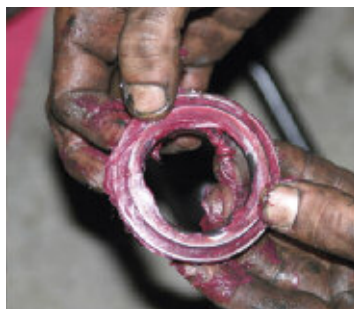
Fig 11 - Repacked bearing ready to install into hub.
