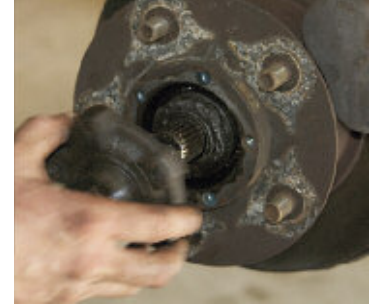
Fig 3 - Pulling drive member off with bolts removed.
