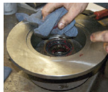
Fig 15 - Install inner bearing and new grease seal. Note: A round drift can be used to install the seal; be careful not to damage when installing.
