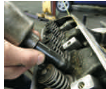
Fig 7 – Head bolt removal with 5/8th socket.
