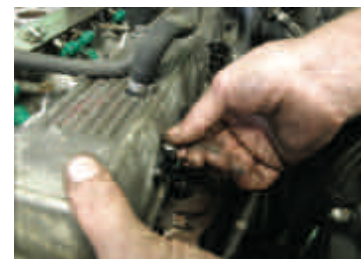
Fig 3 – Valve cover removal.
