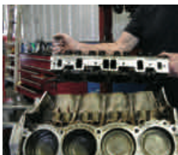
Fig 10 – Exercise care placing cylinder head and head gasket onto engine block.
