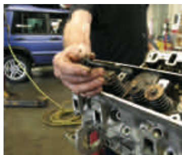
Fig 12 – Installation of new lightly oiled cylinder head bolt.
