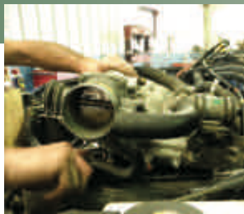
Fig 2 – Upper intake plenum removal.
