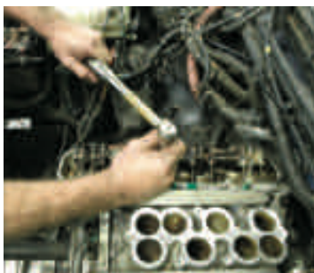
Fig 16 – Reinstall the lower intake manifold.
