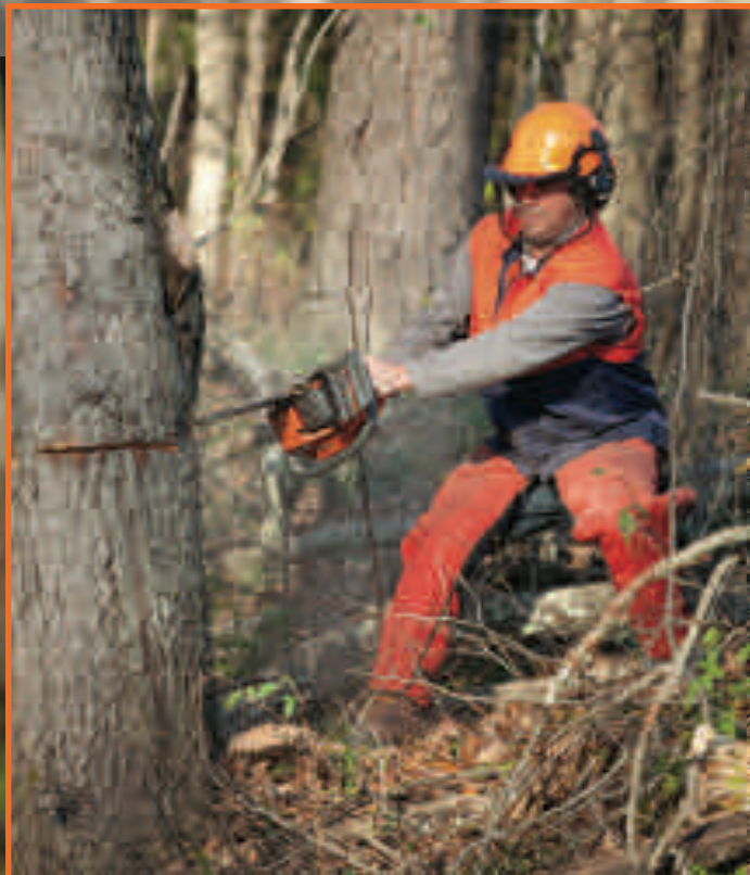
Photo upper left: Performing a plung cut to sever all fibers except hinge and trigger. Lower left: Final cut snipping the trigger.
