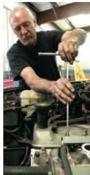
Fig 17 – Jeff White tightens the valve cover bolts.
