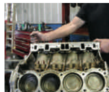
Fig 11 – Cylinder head seated using locater dowels.
