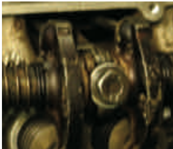
Fig 6 – Remove four bolts securing rocker shaft.
