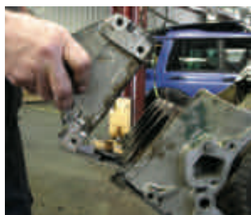
Fig 8 – Removal of the cylinder head. Use care to avoid accidental nicks on the aluminum mating surfaces.
