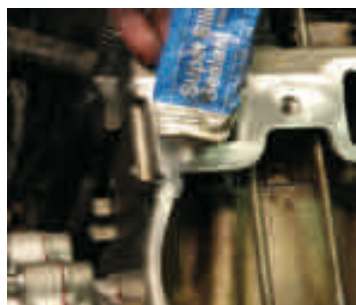
Fig 13 – Application of clear RTV silicone sealant to cylinder head to engine block corner.
